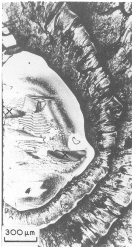
Figure 2 A light micrograph of the fracture surface of a specimen of PSA fractured at 293 K.
