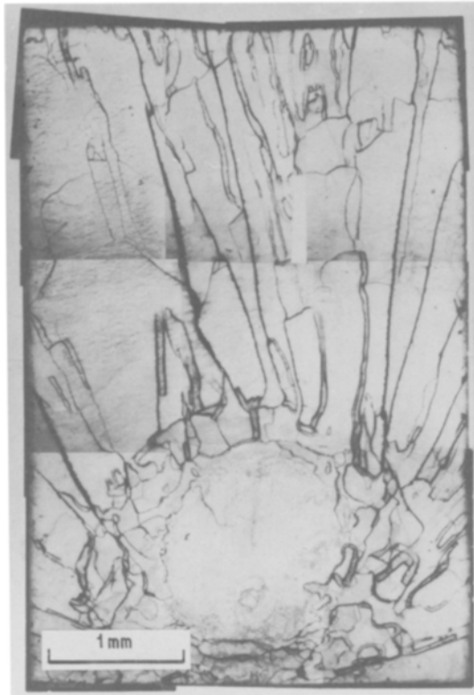
Figure 14 A light micrograph of the fracture surface of a specimen of PSB extruded prior to compression moulding.
